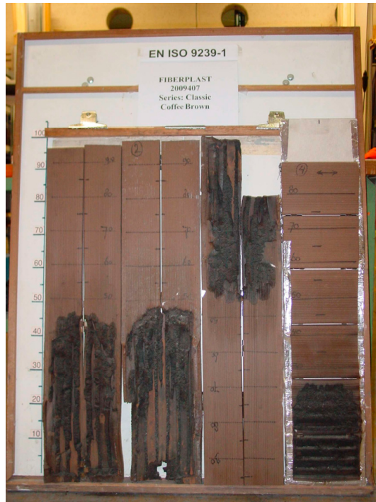
Specimens type Coffee Brown after testing
