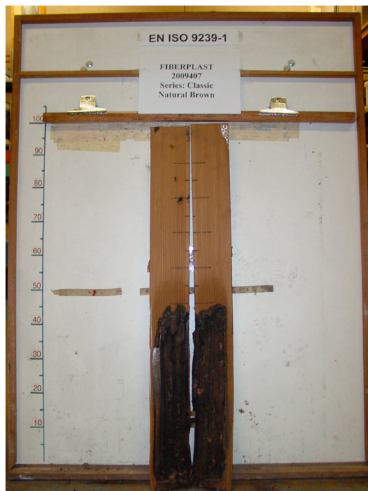
Specimens type Natural Brown after testing
